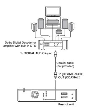
Connect the unit and a Dolby Digital Decoder or an amplifier with built-in DTS using an optional coaxial cable.
